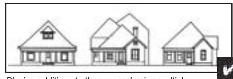
Placing additions to the rear and using multiple rooflines to break up the mass helps to minimize the impact of the second story addition to the center house.
